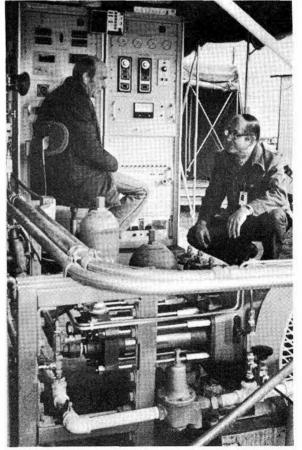
NORB SISKA (2166) contributed programming and automation of computer control to Deep Steam project. trol systems for the Deep Steam Project are the work of Jim Gover's Energy Subsystems Division 2165. The downhole instrumentation package, which measures and controls pressures, flow rates and temperatures, is five inches in diameter and 15 feet long. It is designed to operate continuously in an environment around 500°F.
